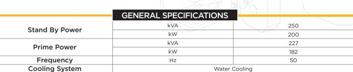
1) Standby power: The max power available during a variable electrical power sequence, under the stated operating conditions, for which a generating set is capable of delivering in the event of a utility power outage. Overloading isn't permissible.
