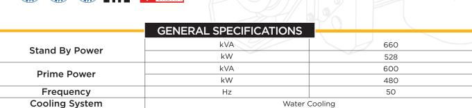
1) Standby power: The max power available during a variable electrical power sequence, under the stated operating conditions, for which a generating set is capable of delivering in the event of a utility power outage. Overloading isn't permissible.
