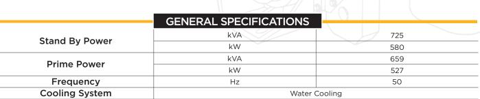
1) Standby power: The max power available during a variable electrical power sequence, under the stated operating conditions, for which a generating set is capable of delivering in the event of a utility power outage. Overloading isn't permissible.
